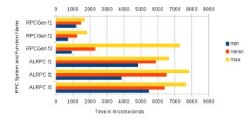
Fig. 3. Comparing ALRPC system and RPCGen system where server and client are on different machines and network bandwidth is approximately 38Mbits/sec. Time shown in microseconds measuring call completion
