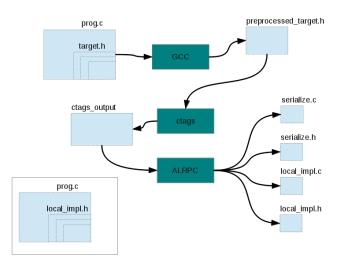
Fig. 2. Static control flow of ALRPC tool chain
