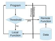
Fig. 1. Decision to move data to local server or to use remote function is based on threshold (Figure grounded in GDAL use case)
