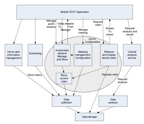
Figure 2: High-level functionality architecture of HCAT
