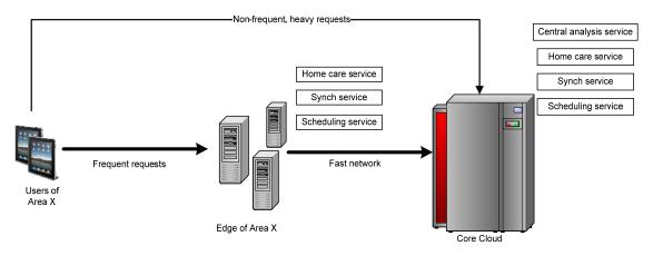
Figure 3: HCAT deployment architecture
