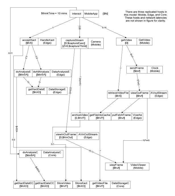
Figure 6: LQN model of the HCAT System. Parameters such as \$hXD are defined in the text.
