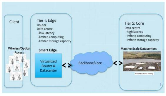
Figure 1: Extended cloud architecture (taken from [2])
