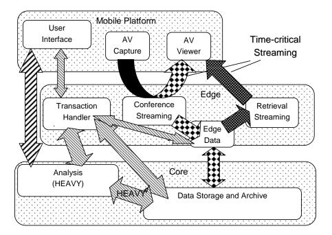
Figure 5: Information flow for the four classes of operations, indicated by shadings
