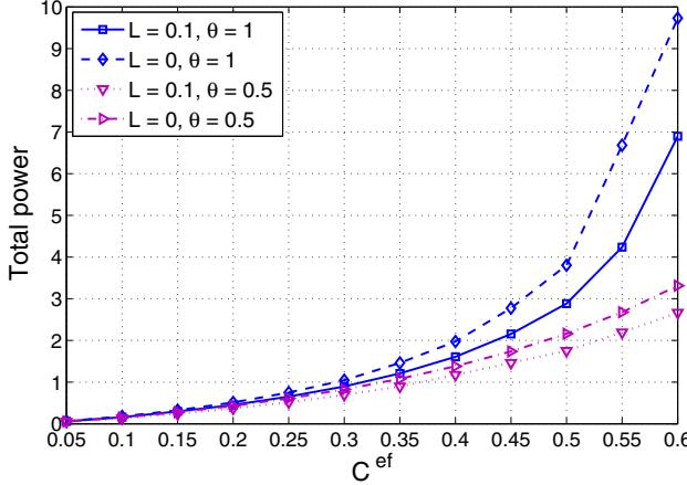
Fig. 1. Total power consumption versus capacity requirement  $C^{\text{ef}}$ .
