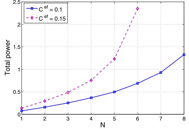
Fig. 2. Total power consumption versus number of users  $N$ .
