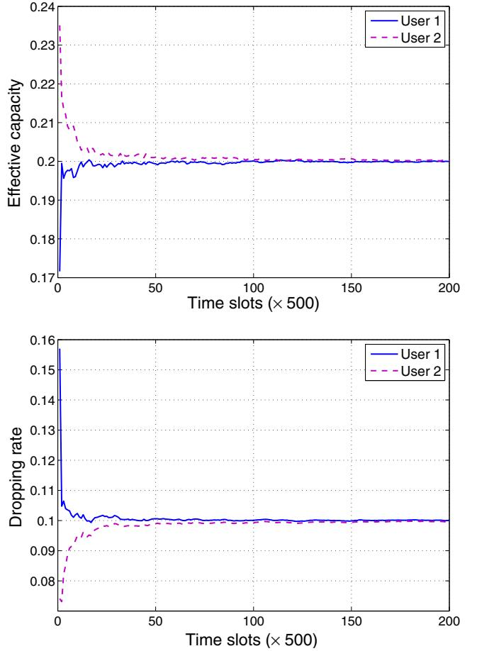
Fig. 4. Convergence of the dropping rate and effective capacity.
