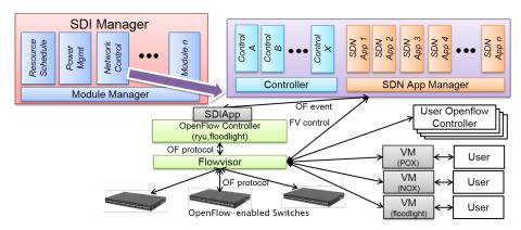
Fig. 3. SDI manager design and an expanded view of the network control module
