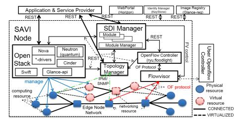
Fig. 2. Design of a control and management system for SAVI node [2]
