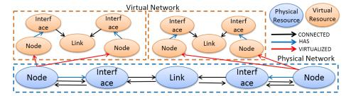
Fig. 5. Graph model example for cloud and networking resources
